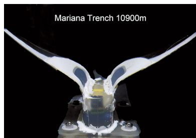
The silicone robot dived to 10,900 meters below the ocean's surface in the Mariana Trench.
